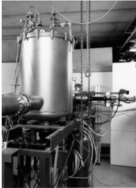
FIGURE 18. Cryostat with detector system at the beam diagnostics test bench (Photo: Achim Zschau, GSI).
