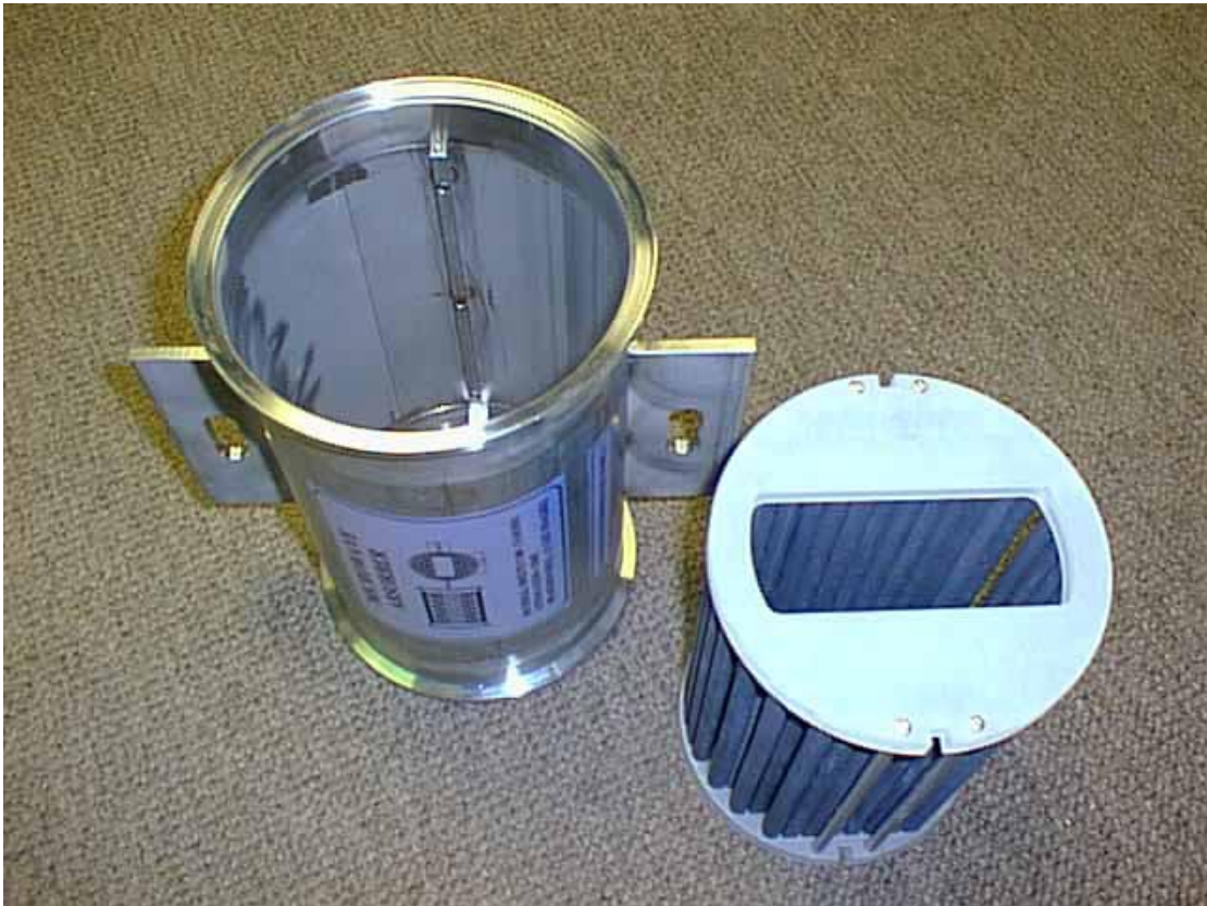
FIGURE 3. Microwave absorber made with an array of ferrite rods.
