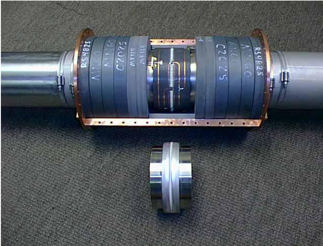
FIGURE 1. Resistive wall monitor showing circuit board and ferrite.
